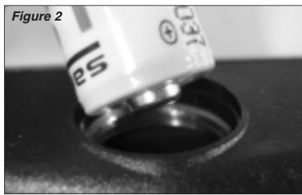
Insert R8 Battery Positive End DOWN .
