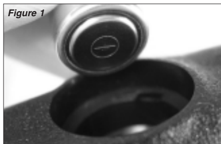
Insert R7 Battery Positive End UP .
